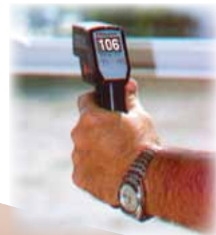
Meter registered 106°F on an eastern exposure window with no film.
